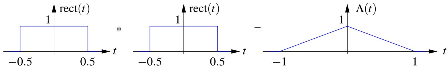
$$\Lambda(t) = \text{rect}(t) * \text{rect}(t) \circledcirc \text{Sa}(\omega/2) \cdot \text{Sa}(\omega/2) = \text{Sa}^2(\omega/2)$$
