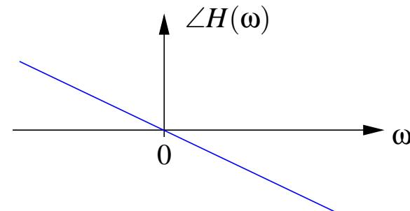
The transmission system must have a constant magnitude response and its phase shift must be linear with frequency (resulting in the same delay of all frequency components of the input).
