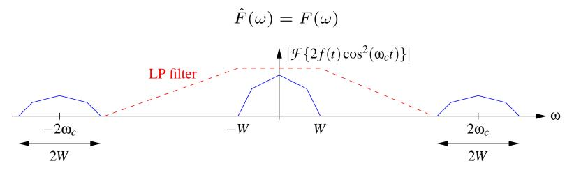
The oscillators at the transmitter and receiver have to be synchronized, i.e. the carrier frequency  $\omega_c$  as well as the phase must be identical (coherent demodulation).
