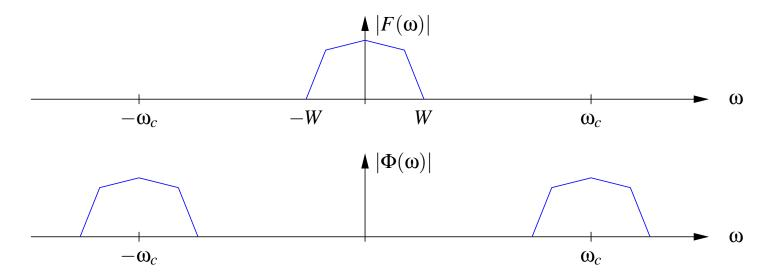
• Efficient antenna design: size is at least  $1/4^{th}$  of signal wavelength  $\Rightarrow$  antennas for lowpass signals would be too large (f = 3 kHz,  $\lambda = 100,000 \text{ m}$ ).
