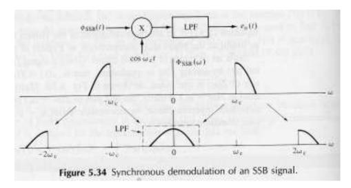
Synchronous detection, analogous to DSB-SC
