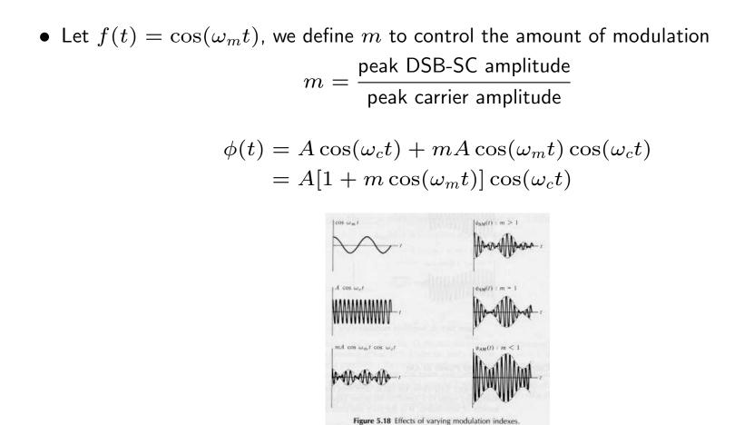
• percentage of modulation for DSB-LC signal with sinusoidal modulation
